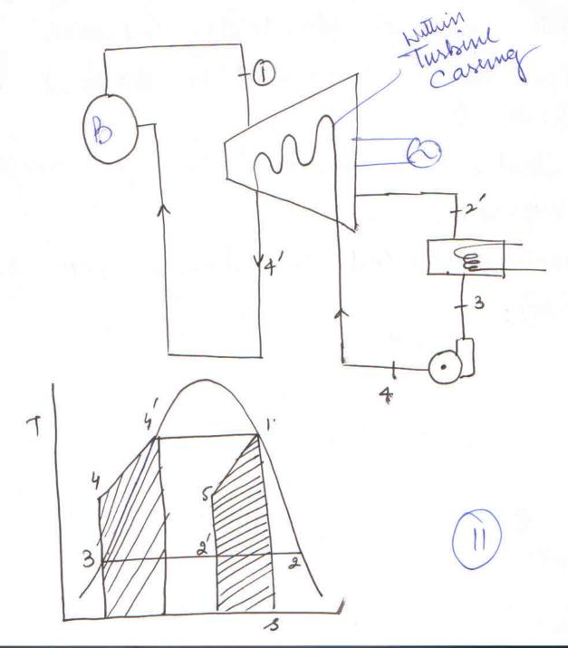
$$Q_{1} = h_{1} - h_{4} = T_{1} (S_{1} - S_{4}')$$
