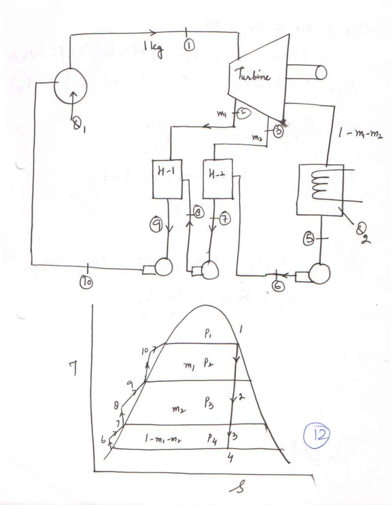
$$WT = (h_1 - h_2) + (1 - m_1)(h_2 - h_3) + (1 - m_1 - m_2)(h_3 h_4)$$
